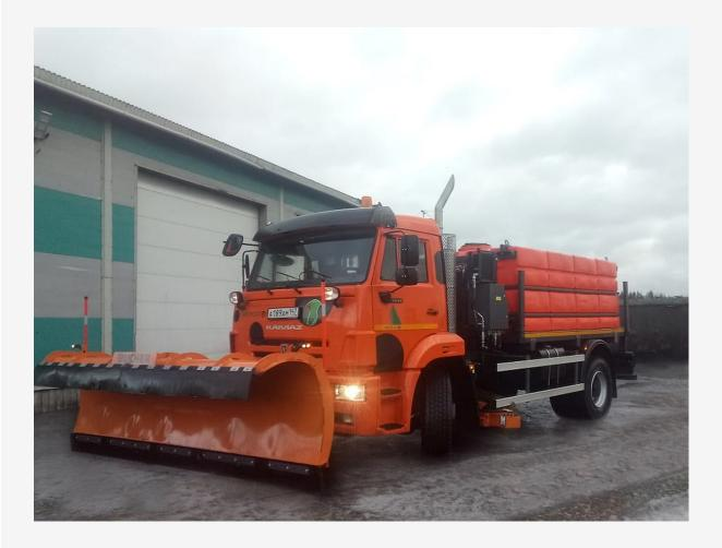
Equipment can be operated in the course of machine motion. An operator can regulate intensity of sweeping by changing the contact surface area. Additional side lights and cat's eyes allow for operation in periods of darkness.
